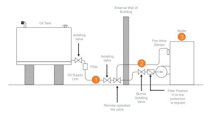
If the temperature in the fuel burning appliance exceeds the temperature range appropriate for that valve, the liquid inside the capillary expands and causes the valve to shut down, cutting off the supply of fuel to the appliance immediately.
