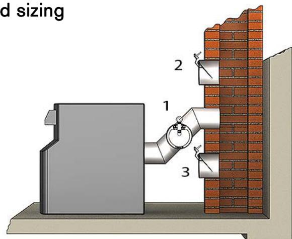
By adjusting the counter weight, the draught regulator can be set to open at different negative pressures. An instruction sheet, included with every draught regulator, shows how many mm to adjust per Pa (negative pressure). All Tigerholm draught regulators are factory adjusted to 10 Pa. The typical value for a home installation is 10 Pa for over-burning, oil and gas boilers. Standard values for other boilers like ceramic and under-burning boilers are 17-25 Pa.
