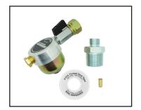
Designed by Atkinson Equipment, featuring an isolation valve, 52 micron nylon filter element, 1" BSP male tank-fitting adaptor, PTFE tape, and a backnut to lock the filter in the correct orientation once the adaptor has been tightened.
