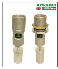
Designed to act as the fill point on both metal and plastic diesel tanks. The Filstop physically closes the inlet to the tank should the fuel level reach its maximum during delivery. This prevents the tank from being overfilled or bursting and hence reduces the risk of pollution and expensive clean up operation that might arise from such an occurrence.
