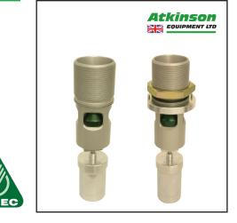
Designed to act as the fill point on both metal and plastic diesel tanks. The Filstop physically closes the inlet to the tank should the fuel level reach its maximum during delivery. This prevents the tank from being overfilled or bursting and hence reduces the risk of pollution and expensive clean up operation that might arise from such an occurrence.
